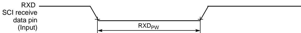
Figure 10-15 RXD Pulse Width
