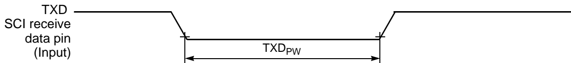
Figure 10-16 TXD Pulse Width
